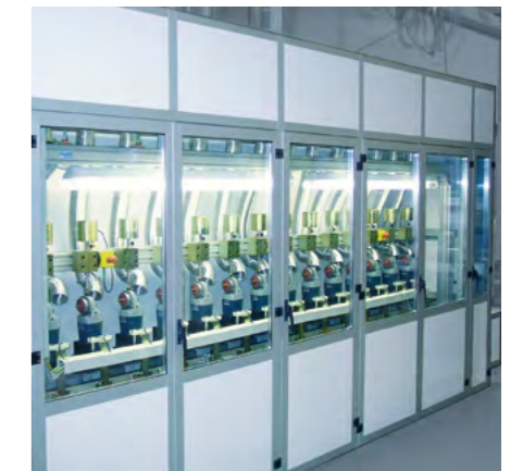
Protective cabinet and noise protection
